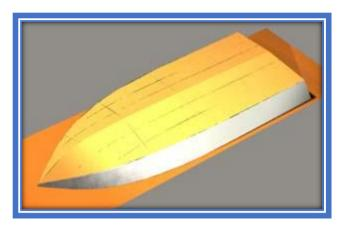
After the cure, we will fiberglass the complete bottom then flips the assembly over and cut all openings in the bulkheads, cut the mid frame from the mid mold and use the floor panels for the deck: no waste of time or materials. The hull will be fiber glassed in and outside with biaxial glass and epoxy, this will produce a composite hull lighter than a fiberglass boat but much stronger.
