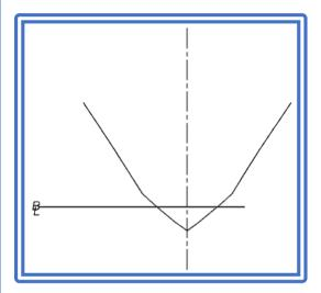
Step two: Mark the height of the center, draw the curve of the deck.
