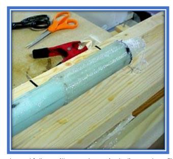
The sleeve covers the reinforcements and should be stretched as much as possible.
