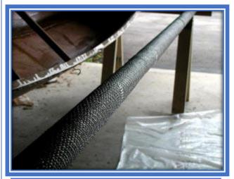
Again, tension is important, pull the sleeve as tight as possible.
