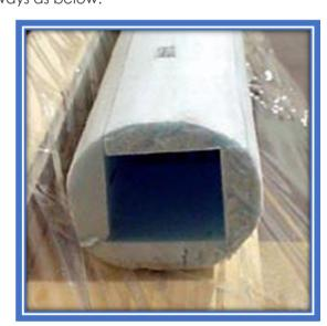
Oops, in this picture we did not grind enough foam to compensate for the mast step reinforcement.
