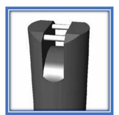
Build those parts from carbon fiber tape or tow with some UHMWP or SS bushings where needed. UHMWP means  $\dots$  (See building notes for complete text)
