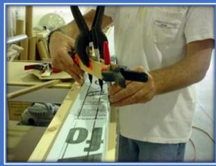
With the sides of the gauge pressed against the sides of the box, the gauge will draw a perfect taper.
