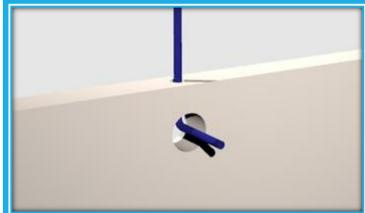
At the top, the painter (line) can be tied to a cleat but we show a simple and elegant alternative. The keyhole shaped plate can be made from brass or hardwood or plain plywood epoxy coated. Several knots can be made in the painter, each corresponding to different CB settings: completely down, halfway, all up etc.
