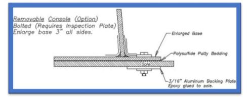
Important: It is not visible on the drawing, but the fiberglass lamination extends under the bolts and washers.
