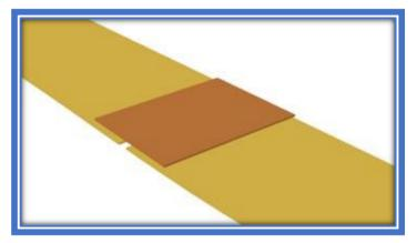
Cut the frames from the dimensions given on the plans. Assemble the sides around mid-seat frames with the butt block as a locator.
