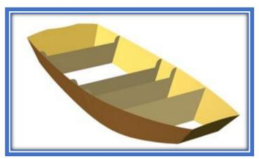
Cut the seat tops from the dimensions given on the plans. Install the seats tops DRY on cleats (see construction drawing). This will allow us to check and, if necessary, correct the symmetry of the hull. Install the rubrail.
