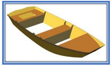
Flip the "boat" over and install the bottom panel on the hull. The bottom panel butt block fits exactly between the mid frames. Stitch or duct tape the bottom to the sides, flip over again.
