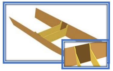
Install the transoms between the sides. The building notes included in the plans package explain all this in detail.
