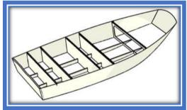
6. Check diagonals. This is a very important step: the diagonals must be equal within (5 mm). Diagonal means a distance between one corner of the stern transom and the opposite corner on the bow transom. No need to measure, use a line. Once the boat is square, secure a diagonal by fastening a batten across the boat as shown.
