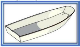
9. Build the inside seams around transoms and along chines. Cover inside with biaxial fabric. Reinstall stringers, tab to hull.
