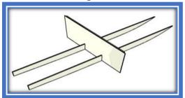
2. Note that we epoxy glue the seat battens to the frames at this stage. Without them, the frames would not be sufficiently stiff to shape the hull. Install all other frames and the transom on the stringers except for the forward frames. Not shown on the picture are the motorwell sides between the last frame and the transom. They are required for the transom angle.
