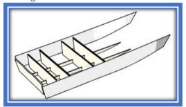
4. Install the bow transom between the side panels. This will require supporting the bow transom with some blocks, supports not shown.
