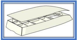
8. Build all outside fiberglass seams and fiberglass bottom. Sand, prime and paint. Flip the hull over, install rubrail. Remove all inside framing including the stringers
