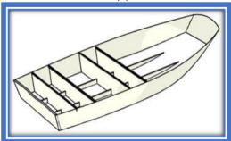
5. Install the forward frame with support. Optional: install the longitudinal bulkhead under the casting deck (not shown).
