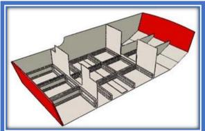
**Step 9:** Install sole panels in cockpits and inside, epoxy glued on framing, FG seams all around perimeter on upper side.
