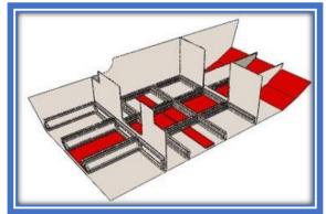
(Butt blocks are used on the flat part of the bottom, fiberglass seams at the bow. Specifications are given on the plans)
