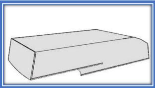
Step 12: Install strakes, epoxy glued. Roll over.
