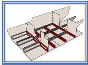
**Step 7:** Install bottom butt blocks between framing. Install the two bow bottom panels and build FG seams at bow bottom panels.
