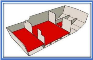
Step 10: Build inside accommodations structure. Install rubrails.
