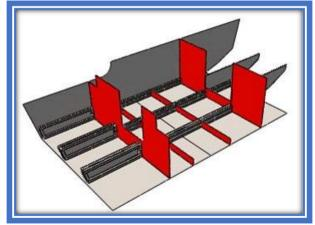
**Step 6:** Epoxy glue longitudinal and transversal framing to bottom panels including side panels.
