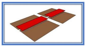
Cut the longitudinal butt blocks. Epoxy glue
