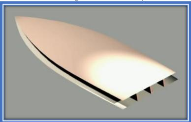
**Step3:**Cover the keel sides, build fiberglass seams.
