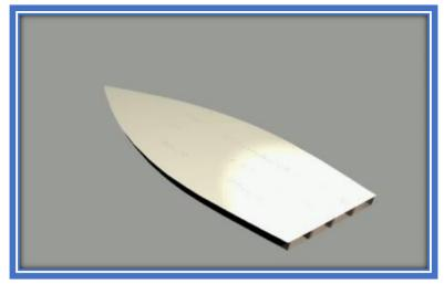
**Step 5:**Install the mid mold on the cockpit sole.
