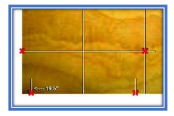
The seat is 10.125" above the bottom (1' 0-1/8"). Using the same method, we draw a line at that level.
