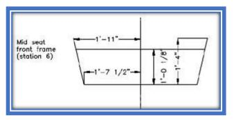
What we are going to do next is draw the outline of the frame using the dimensions from the plans, It is very simple: just some straight lines. Start by scribing the center line at 23" from the edge of the plywood, no waste. To draw a perpendicular, use a square or easier, just measure 23" on each side of the plywood and draw a line.
