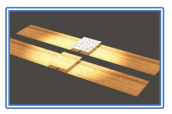
The fiberglass splice shown on top uses one or several layers of fiberglass tape in epoxy instead of a butt block.
