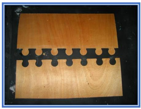
To assemble a puzzle joint is simple: • work on a flat surface covered with a plastic sheet
