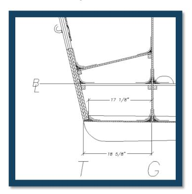
**Step 3**: Understand where we measure from: the origin. In the case of the DE23, our origin for the dimensions is the lower tip of the transom, outside face. Since the stringers stop on the inside face, we must subtract the thickness of the transom. The distance from the lower tip of the stringer to the motorwell bulkhead is 17-1/8". Note that at this point, we don't worry about the thickness of the bulkhead.
