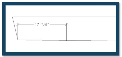
**Step 5**: Draw a second frame location. Note that I did not worry about any thickness, I just drew a line. This makes sense if you look at the plans: the dimension lines show clearly that you measure from the previous location line. Please do not think of the thickness or the depth of the notches at this point, keep it simple, location marks only. Mark them with the frame letter.
