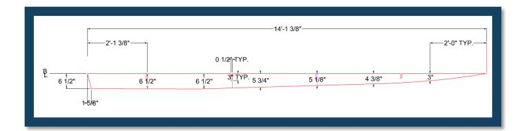
**Step 2**: Look for the frame spacing. This should be on the Stations drawing in your plans. Note how each frame is identified by a letter, T being the transom.
