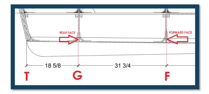
**Step 8**: Mark the depth of the notches. In most cases, 3" (75 mm) will be fine but there is no absolute rule. Let's do it at 3". Draw a line parallel to the sole (the upper face of the stringer), 3" down.
