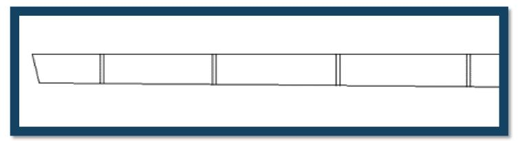
The dimension lines on the plans clearly show where we measure from. In this case, for the DE23, the first location, line G, refers to the REAR FACE of the frame G. You know the thickness of that piece of plywood: add it forward of your location line. The second location, line F, is to the FORWARD FACE of the frame. Add the thickness behind that line, towards the stern. There are reasons why we do not always use the same face. Proceed the same way for all your frames.
