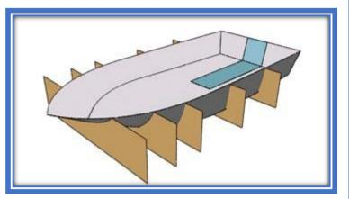
Install stringers and floor frames Install the stringers and floor frames in the hull shell. This can be done in one or two steps depending on your vacuum bagging skills and equipment. If you proceed in two steps, install the stringers first. The stringers must be in one piece with the floor frames between them. The stringers are capped with carbon fiber. See the lamination drawing for specifications and stack order.
