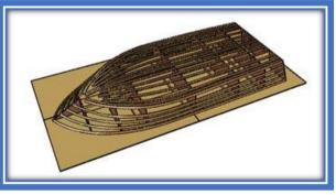
The molds can be made of particleboard. They should be sufficiently thick to take screws for the slats. Take the molds dimensions from the stations drawing.
