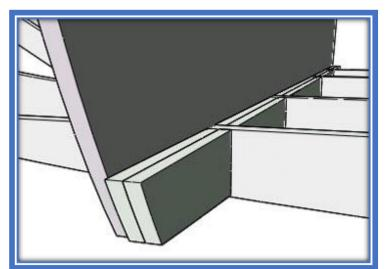
not sit on a foam pad. Build a ?" fillet at the seams with structural putty. Keep in mind that we will cut the tunnel and false transom openings later. There is no tabbing or fillet where we cut.
