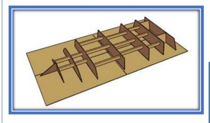
Set all your flat parts aside and start the jig assembly. Build the jig (male mold). The PH15 hull is assembled on a traditional slat jig. That type of jig is sometimes named a ribband mold. It is made of molds covered with widely spaced longitudinal battens.
