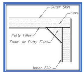
glued to the sheer with epoxy putty and tabbed all around inside and outside. The finish and fairing are done the same way than on any other fiberglass boat. A glued vinyl rubrail is appropriate for this boat. The topside foam will take the screws until the epoxy glue cures. The same applies to other small parts like a toe rail.
