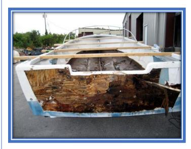
The previous "rebuild" included a bunch of mats laid into the bottom. All this mat and the remaining roving from the stringers (which did not peel off) will be ground out. New heavy biaxial cloth (1708 or 1808), will be laid into the hull using epoxy resin. This will reinforce an almost 30-year-old skin as well and give us a very good base/foundation for the new stringers and frames.
