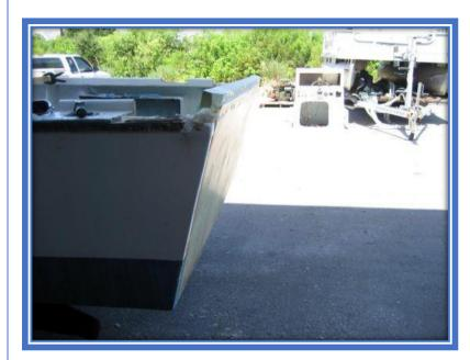
We put in the first 2 layers of inside transom skin. First layer is <u>1708</u>, second is <u>DB1700</u>. The inside skin will be 4 layers total of <u>17 oz. Biaxial glass</u>. The first layer has mat (1708) because the mat helps conform to any uneven spots in the fillet. Subsequent layers will not have mat as it will just use more epoxy and not add strength.
