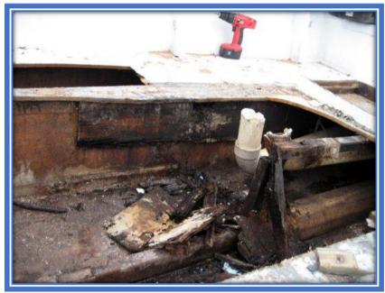
We are going to take extra precaution to ensure the shape of the hull doesn't change before we get new stringers and frames installed. Like pulling a brand-new hull from a mold, unless there is some structure in the hull, it could "oil can". The next step is to build a cradle to support the shell and keep her strait and fair. While it looks fine now, a little extra work in building the cradle is worth the peace of mind; especially when you plan to put a lot of work and money into the boat.
