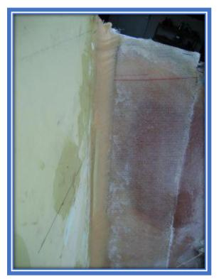
After 15 minutes or so, the fillet is firm but not hard. At this point we lay in the pre-wet 1708. Because the fillet is not hard, you will be able to push the glass into the fillet making for a very clean lamination – no air bubbles. A second layer of DB1700 was wet out on top of the 1708. DB1700 (17 oz. without mat) wets out much easier than 1708, so you can do it on the part – no need to wet out the back side before placing it.
