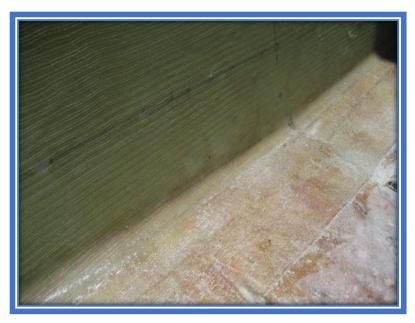
All the inside layers will be overlapped by 3"-4" working up the hull. Working wet on wet saves time and makes for better laminations. In this case we should have gone ahead with the last 2 layers, but time did not permit.
