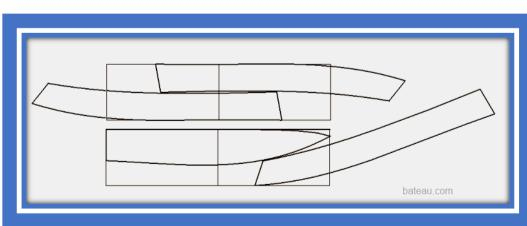
The hull side panels are at the top, the bottom is below it. We show only the hull skin panels but as you can see, to enlarge that boat by only 1" will almost double the amount of plywood required with the added complication of moving the panel splices to the correct place. They can't be at an extreme end. The
