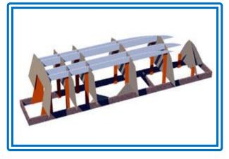
The bow mold is optional. The bow shape is created automatically by the planking, but a bow mold will help to bend and secure the panels. Braces are generally not required since all parts are locked in place, but they will not hurt: we show one vertical, one horizontal, use none or as many as you want.
