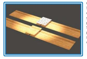
Once the jig is ready, cut the panels for the sides and bottom. The dimensions on our expanded panel drawings are very accurate so there is no need to use a safety margin. We suggest starting planking with the bottom panels. Cut the panels and use fiberglass splices to join the pieces of plywood. The plans or building notes specify the type of glass to use. The picture shows a butt block at the bottom and a fiberglass splice at the top. Note: No butt blocks needed if puzzle joints are used.
