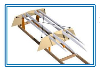
Install inside stringers first. In some cases, the stringers fit in notches in the transom framing. If not use temporary cleats. Outside stringers are fitted next. Check diagonals as shown: the distances must be within 1/8" (3 mm).:
