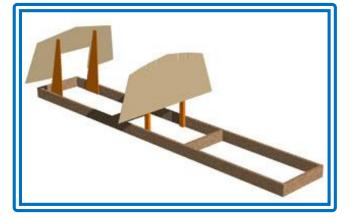
Before installation on the jig, we should frame the transom, cut the outboard well, and install the outboard clamping board if applicable. Build your transom as shown on the plans, flat on the floor. On the jig, the transom is installed at an angle. The plans show that angle and also show a triangular brace that automatically produces that angle. Cut the triangular brace and install it on the jig. The distance from the origin and the height are on the plans, same as for the molds.
