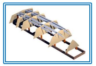
Add molds starting from the transom. They should fit in the stringer's notches. Some optional molds and bracing can be added at this time
