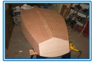
When installing the side panels, beware of longitudinal alignment. If the side panels seem not to fit, slide them back and forth. A small movement will bring everything into alignment. As is typical with our method, allow the panels to float, meaning that we try to attain fairness first. Use as little fasteners as possible and do not pull the panels against the frames unless absolutely necessary.
