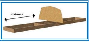
how far that mold is located from the origin lengthwise. Measure that distance on each of the strong backs and scribe a line. I hope that you saw on the plans that we measure from a specific mold face, forward or stern side. Align that face with the line, not the other one. Center the mold on the strongbacks. All that is needed to find the final position of that first mold is the height.
