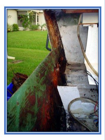
Once the old plywood and putty are removed, make a template of the transom using cardboard or cheap plywood (or anything else handy). You will use this template to cut your transom core and to draw/cut the wide fiberglass pieces that will make up the new inside transom skin.
