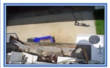
Now you must completely remove the old plywood core. A reciprocating demo saw, grinder, hammer and chisel are good to have. If you have an air compressor, a small air hammer is a good investment. Be careful to not inflict too much damage to the outside fiberglass skin. If you do damage the outside skin it is not a big deal, but you will want to reinforce it with a layer of fiberglass before the new core is installed (more on that later).
