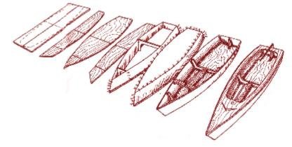
First generation stitch and glue boats were made of plywood parts glued with fiberglass tape and resin. The panels were stitched together with copper wire to keep the assembly together during the resin cure. The wire was removed later. Many stitch and glue designs still rely mostly on wood framing for structural strength and are not true composite boats.
