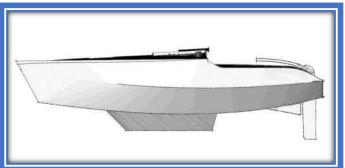
The rudder moves forward on the new transom and rotates in a slot just like in the VG20. The rudder gets better support and is will give better control in it's new location. It can move up and down for shallow water sailing. The skeg became slightly larger for better tracking. The split backstay is connected to chainnplates mounted on the new transom. The backstay moves to the new transom. This will limit the amount of roach in the main but that is perfect for long distance sailing.
