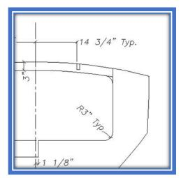
Also, the location and size of the longitudinal roof framing was not clear. They are 1" X 2" [25 X 51] on edge and 14 3/4" [375] from centerline.
