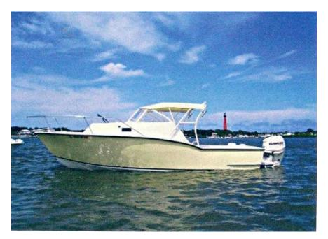
The CX25 is an offshore boat based on the Carolina Sport Fishing boats lines. The hull is identical to our CS25. We offer two hull materials option: foam sandwich or plywood-epoxy-fiberglass composite.
