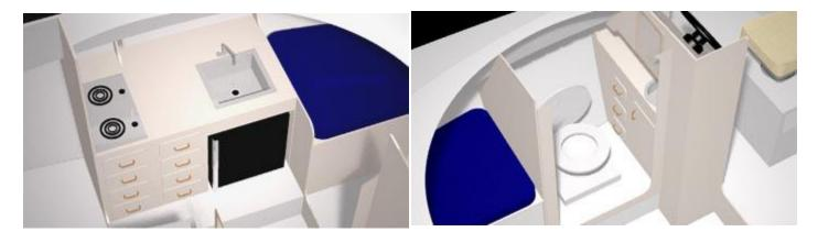
The head is isolated from the cabin by a real door, not a curtain. The galley can accommodate a fridge, sink and stove. Headroom is close to 6' under the companion way hatch and there is comfortable sitting headroom over the vee berth. There is ample room for tanks: fresh water and waste.
