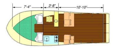
The cabin layout is typical of that type of boat: a generous vee berth with a drop down table (not shown) followed by a galley unit on the port side and a head on the starboard side.
