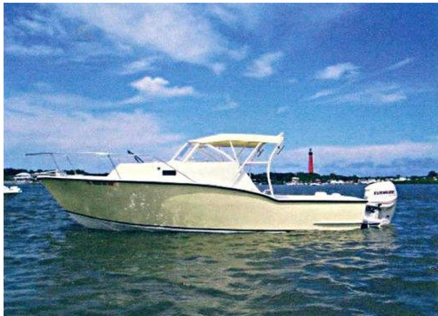
The CX25 is an offshore boat based on the Carolina Sport Fishing boats lines. The hull is identical to our CS25. We offer two hull materials option: foam sandwich or plywood-epoxy-fiberglass composite.
