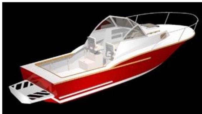
The self-bailing cockpit is more than 28" deep at its lowest point and cockpit depth standing on the casting deck is more than 30", an important safety factor.
