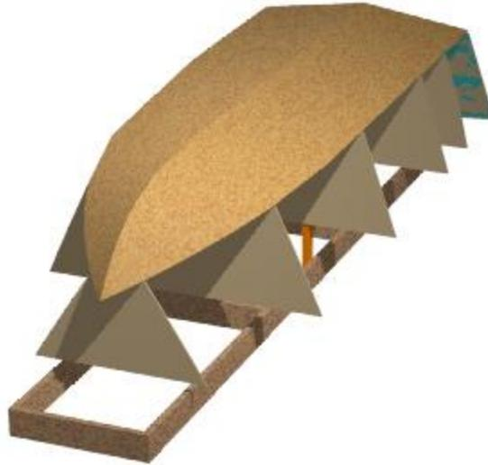
Our jig system is very uncomplicated, self-aligning and economical since we use the internal framing of the hull as molds. Our jig does not require all the precautions, alignments or even a perfectly flat floor that are a must for traditional boat building.
