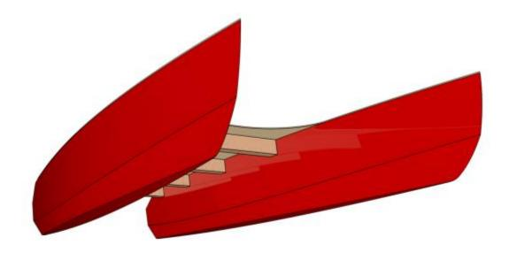
The hull section is made of five panels with a narrow bottom. This is the closest one can get to a low drag cylindrical section with a limited number of plywood panels.
