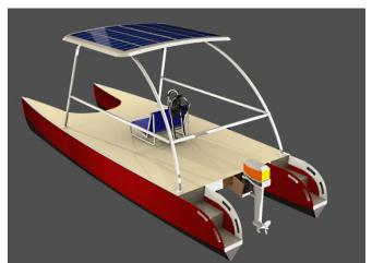
The plans include dimensions and specifications for the bracket and the building notes explain how to adapt the bracket to different shaft lengths. The minimum shaft length for a single motor is 20".
