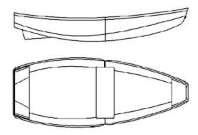
Less than 6' (1,80m) long when nested but almost 11' assembled, this dinghy is not only ideal to store on deck of a larger boat but in the back of a pickup truck or for the winter in a corner of the garage. The two parts are locked together by the removable center seat and secured by a set of simple bolts with wing nuts. She rows well but can also be fitted with the same sprit sail than the D4 and PK78. She can take up to 4 HP: the plans show transom reinforcements for outboard use.
