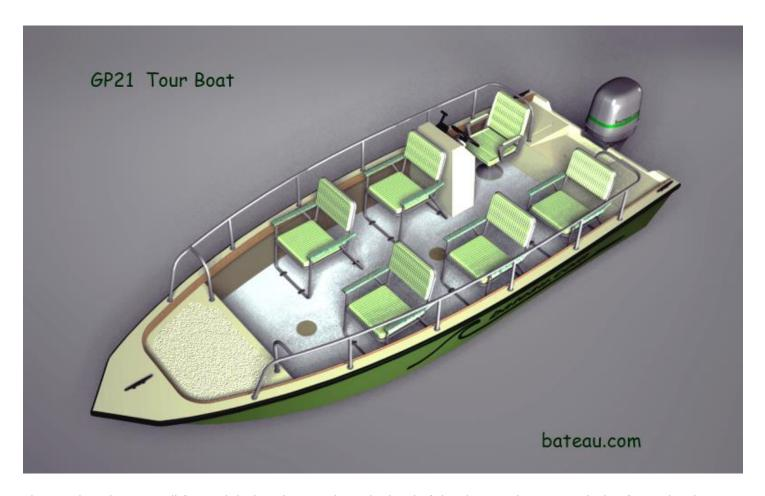
The tour boat has a small forward deck with gunwale at the level of the sheer and a casting deck a few inches lower: boarding from the dock is easy and safe.
