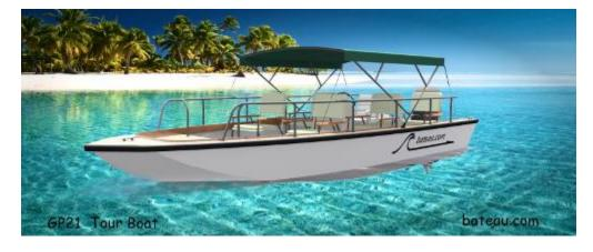
The GP21 is a wide garvey hull with good planing characteristics, stable, roomy and smooth running in a moderate chop. The hull is based on a proven work boat shape. There are several companies producing variations on that type of hull, mostly in aluminum.
