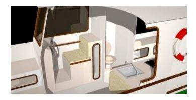
The aft cockpit can be enclosed by a canvas tent. The flat sole is 5 'x 6'-3" (between the benches), the width of a queen size bed! Perfect for an inflatable bed. The canvas cockpit enclosure is supported by the boom but a standard pontoon boat enclosure will fit perfectly. Those can be bought at a very reasonable price from most marine stores. Windows may be replaced with screening, or left open.
