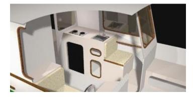
The cabin has **standing headroom**. We recommend a Porta Potti type head to avoid complicated plumbing. There is storage everywhere and the boat has sufficient capacity to fill all those places with fishing gear, beach and camping equipment etc.
