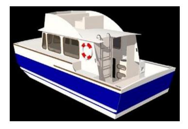
From the cockpit, two steps lead to the foredeck. The gunwales are 14" wide (35 cm). The foredeck is fitted with an hatch over the forward cabin and can also be equipped with bow rails.
