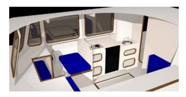
The suggested layout for the galley shows a double burner stove with or without oven, a fixed sink, room for a small fridge and a nice working area.
