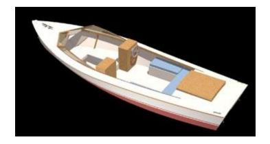
The hull can be built the stitch and glue way, upright with panels folded around the frames or better upside down, using the frames as a jig. See the <u>our building tutorial for a step by step overview</u> of the process.
