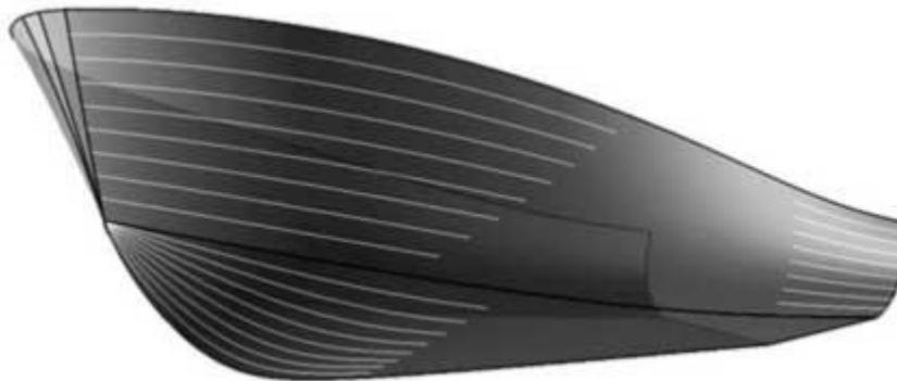
*The picture shows the areas requiring slits in the plywood. That technique is used on several other boats and well proven. It creates a transition between sheet plywood planking and strip planking.*
