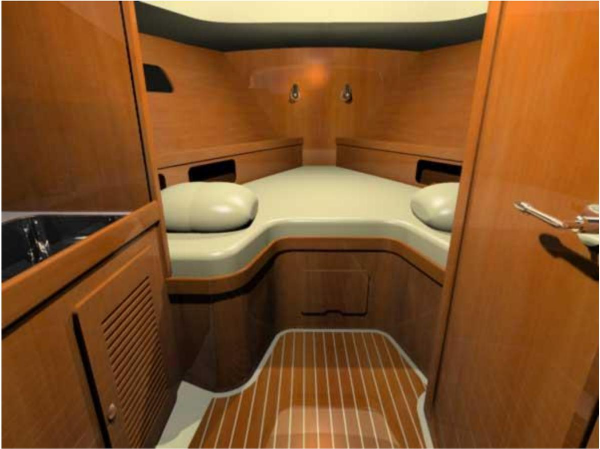
Inside there is a roomy cabin with vee berths 2 meters long (79"), a small but practical galley on the port side and a fully enclosed head on starboard. Freshwater and waste tanks are 26 gallons (105 liters) each and there is room for more.
