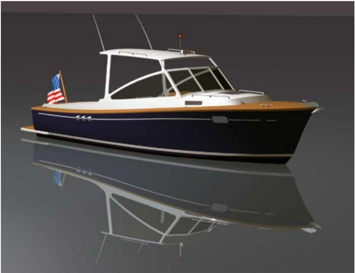
The plans can be customized as long as the builder does not compromise the structure. Seating can be added to the cockpit, the cabin layout can be changed, the hard top can be different but the cabin height should not be increased excessively and if the boat is fitted with a pilot house, it must be kept very light.
