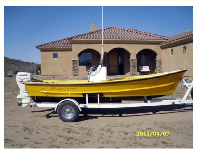
The displacement at DWL is 1,500 lb. (680 liters). The PPI is 298 lb (53.3 kg/cm). A US Coast Guard capacity tag would show max. capacity 4 persons or 650 lb., 950 lb. persons motor and gear. Max. 25 HP with tiller steering, 40 HP with remote steering. It would be very easy and legal to calculate a tag for 7
