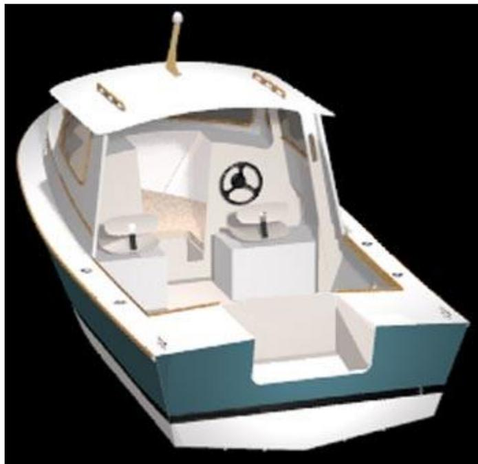
The self bailing cockpit depth minimum 26" with 12" wide gunwales, is another important element of safety. Her PPI is at DWL is 543 lbs (247 kg). Thanks to the freeboard and transom design, she can be rated to a max. capacity of eight persons (USCG) and we recommend engines in the 90 to 150 HP range. While stronger than the typical production fiberglass boat of that size, she is also lighter and does not require as much HP (or fuel) to cruise at the same speed.
