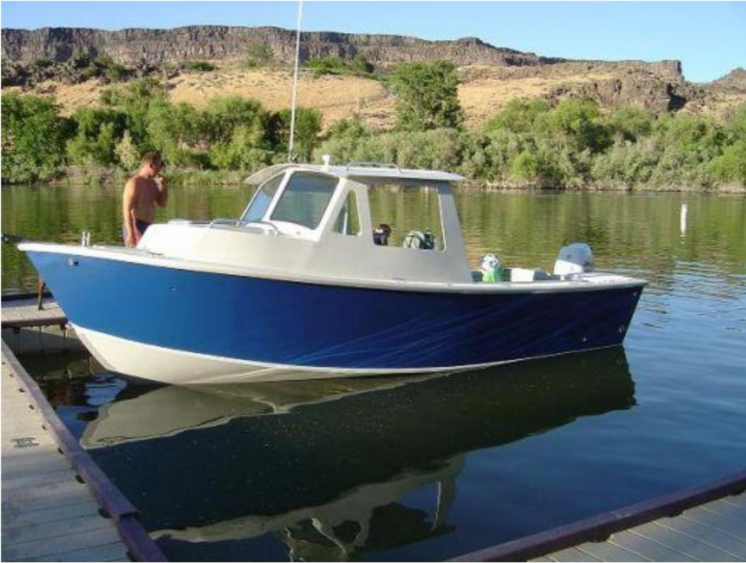
The generous freeboard and the classic sheer are tried and true features contributing to seaworthiness. This boat will negotiate both head and following seas with ease. Lightly loaded, the P21 will require 90 HP to cruise in the low 30 mph range. 125 HP is recommended for a well equipped boat at full load. This boats transom is designed for a standard 25" shaft. The transom can easily be modified to accept other shaft lengths.
