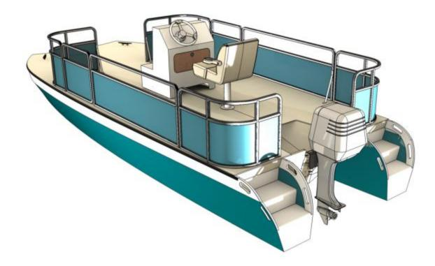
The fine hulls allow this boat to move relatively fast with a small outboard, much faster than a monohull of the same length. With a larger engine, the boat will get on plane without having to push through a steep bow wave: the boat is comfortable at any speed in between. Compared to cylindrical pontoons, the asymmetrical catamaran hulls result in a better water flow between the hulls with less restrictions or wasteful turbulence.
