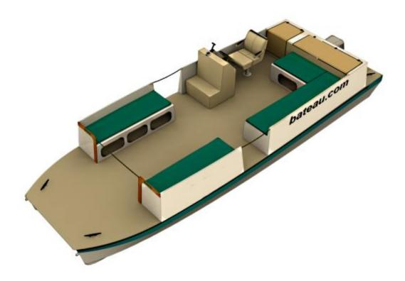
The classic pontoon boat offers a maximum of comfort: no other boat in that size has a changing room that can be fitted with a Porta Potty. The changing room has a low profile under way but when the lid is open, it reveals a curtain running on a rail bolted to the lid.
