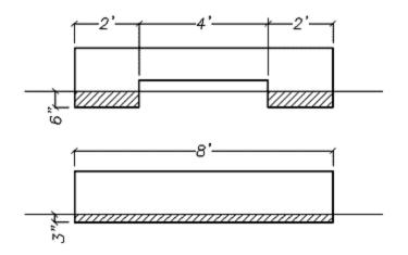
Even if the tunnel is narrower, the cat hull will always need more draft but there is more: a cat structure is more complicated and the hull area is larger, therefore heavier.
