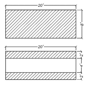
You can see that the catamaran hull as less foot print than the monohull: at equal draft, the cat displaces only half the water of the mono hull and therefore, at equal boat weight will have two times more draft.
