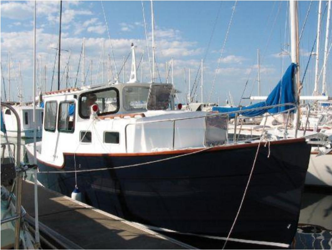
Displacement hulls are typically used for work boats, fishing boats and pleasure boats where moderate speeds are sufficient to fulfill operating requirements.
