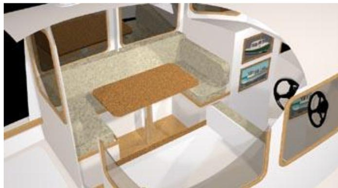
The dinette that will seat four or more and the table drops down to become a double bed. There is room for a cabin heater or even a wood stove with chimney behind the steering station.
