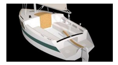
The shallow draft CB and lifting rudder allows access to remote waters and makes launching and retrieving from the trailer very easy.
