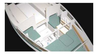
The cockpit is as large as in some 35' sailboats! The total length is just a few inches under 8' and the two benches are 6' long: once can sleep under the stars. There are convenient lockers in the backrests (gunwale). The cockpit and benches are sloped towards the stern and drain easily and fast.
