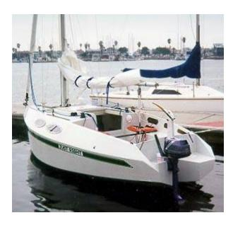
The rigging uses swept back spreaders for better performance, the centerboard version has a profiled CB and less draft thanks to the gain in hull weight and the interior was redesigned for longer berths in the saloon.
