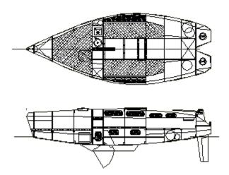
The interior is exceptionally roomy thanks to the raised deck design: 4 full size berths, galley with sink and stove, an optional folding chart table and a dining table that slides under the cockpit. The forward cabin can be isolated by a curtain. A Porta-Potti is located under the V-berth. Roomy cockpit with storage for an inflatable dinghy or raft under
