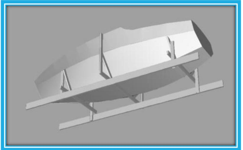
While a true stitch and glue composite hull can be built without any jig or mold, we preconize the use of a small number of partial female molds. Our plans give all the dimensions necessary for these molds.
