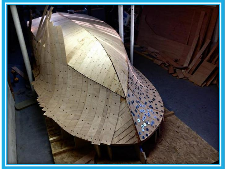
All glue and laminating resin must be epoxy. No fasteners are required: the strips and plywood are installed with staples, often plastic staples like the ones from Raptor. Many builders have used that method to build large replica runabouts. The boats are stronger, stiffer than the originals. They look just as good and require less maintenance. The method is described in detail in the Gougeon book.
