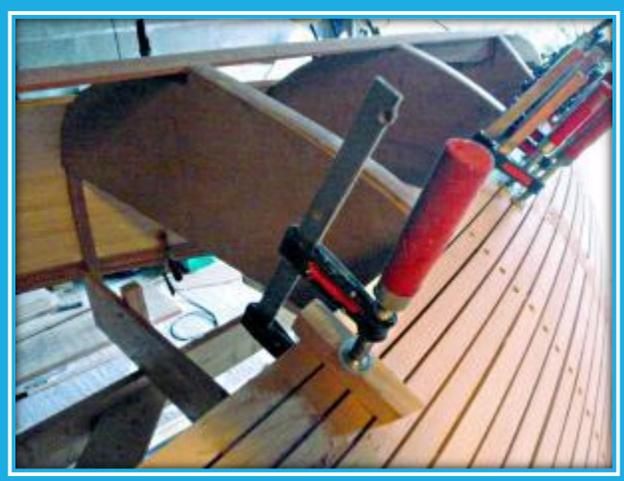
Rarely, the free plans will show a strip planked hull. This is a method in which the framing is covered with thin strips of wood, usually cedar. Many builders substitute plywood strips. In all cases, use epoxy as the glue and if possible, cover at least the bottom with a thin layer of fiberglass in epoxy.
