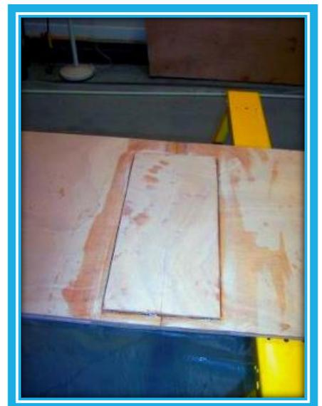
A better method is the **fiberglass splice**. It is somewhat like the butt block: two panels are joined at their edges and covered on each face with fiberglass tape in epoxy.
