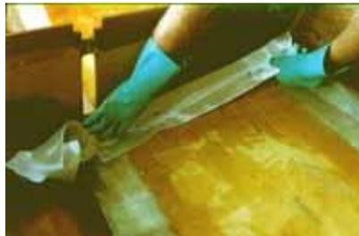
Wet the fiberglass with the resin. It will become transparent while absorbing the resin.
