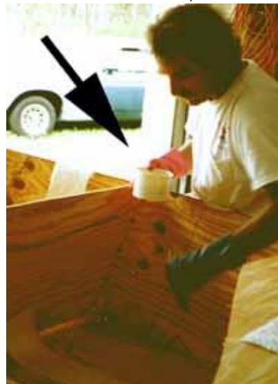
We need some putty to fill the corner first. The putty is made very easily from resin mixed with a filler: micro-balloons, [wood flour](#) etc. It can be applied with a spatula but we describe better methods in our "Stitch and Glue" manual. Note that all surfaces are pre-coated before the application of putty or fiberglass.
