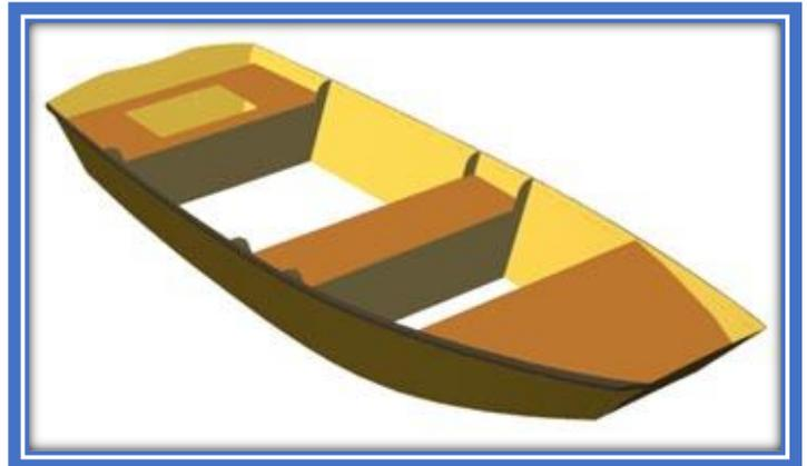
Flip the "boat" over and install the bottom panel on the hull. The bottom panel butt block fits exactly between the mid frames. Stitch or duct tape the bottom to the sides, flip over again.
