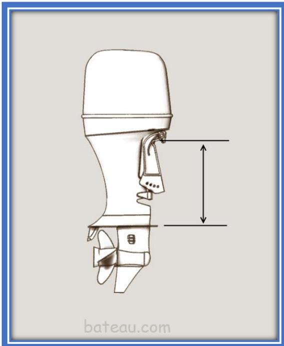
Many small engines, 10HP or less have shafts around 17.5" long (45 cm). Outboards sold for sailboat propulsion often have an unusual long shaft for their size. Very large engines, 250 HP or more, can have 30" long shafts. (from here, I switch to inches only as units. 1" = 2.5 cm).
