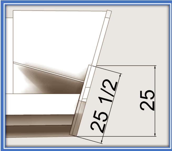
To install a 20" shaft, we do the opposite: cut the transom 5" deeper at the clamp and lower the motor well bottom panel.
