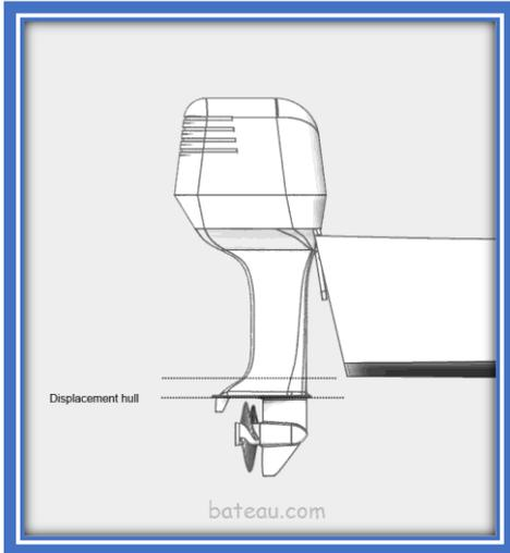
Note that we have not looked at the water line: our outboard prop depth is set in relationship to the hull bottom, not the waterline (power boats).
