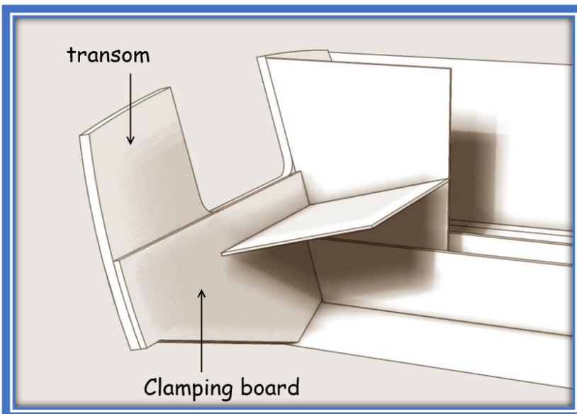
Vertical heights and angled lengths: the difference between the vertical height and its projection is small and can be disregarded when cutting the plywood. That small difference gives us a nice gap for the thickness of the fiberglass. Let's use a large size outboard powered boat with a motor well as an example. The transom is designed for a 25" shaft.
