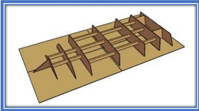
Set all your flat parts aside and start the jig assembly. Build the jig (male mold). The PH15 hull is assembled on a traditional slat jig. That type of jig is sometimes named a ribband mold. It is made of molds covered with widely spaced longitudinal battens.
