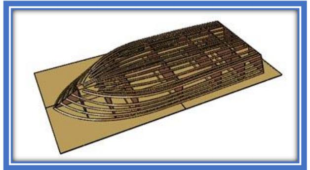
The molds can be made of particleboard. They should be sufficiently thick to take screws for the slats. Take the molds dimensions from the stations drawing.
