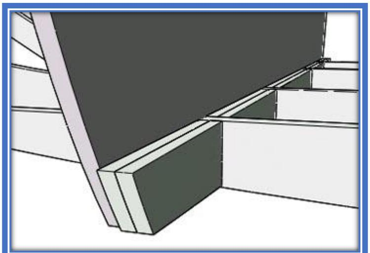
not sit on a foam pad. Build a 2" fillet at the seams with structural putty. Keep in mind that we will cut the tunnel and false transom openings later. There is no tabbing or fillet where we cut.
