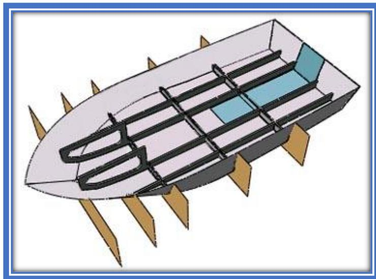
Install stringers and floor frames Install the stringers and floor frames in the hull shell. This can be done in one or two steps depending on your vacuum bagging skills and equipment. If you proceed in two steps, install the stringers first. The stringers must be in one piece with the floor frames between them. The stringers are capped with carbon fiber. See the lamination drawing for specifications and stack order.
