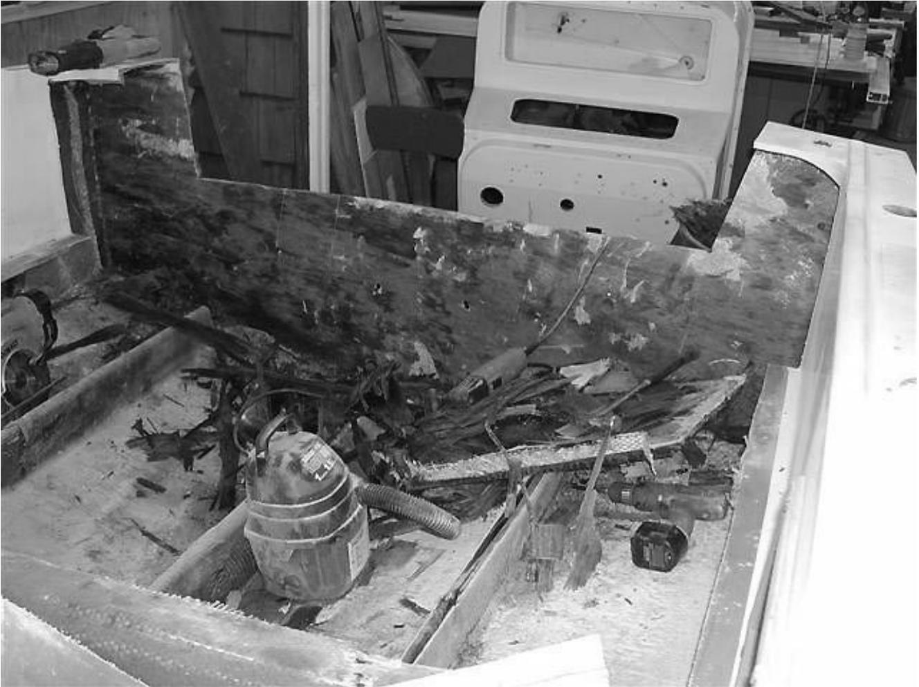
Grind down all the wood to the bare fiberglass. Extend the grinding to the hull sides and bottom at least 8".
