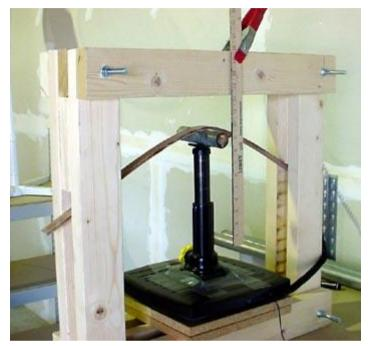
The picture here shows a deflection of 5 (2-1/2"). At that point, the plywood is completely delaminated, but the glass skins are still doing their job.
