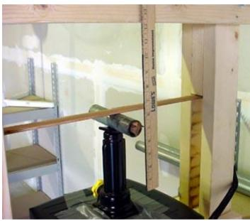
The jack applies pressure to a thin panel sample. We use a steel pipe to distribute the load. The pipe is fitted with a pencil that points to a ruler to measure the deflection. The pressure is measured through the load applied on the scale, all very simple.
