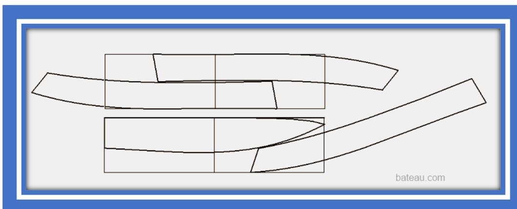
The hull side panels are at the top, the bottom is below it. We show only the hull skin panels but as you can see, to enlarge that boat by only 1" will almost double the amount of plywood required with the added complication of moving the panel splices to the correct place. They can't be at an extreme end. The
