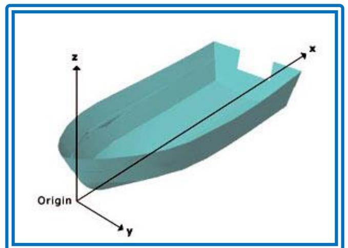
free to raise the imaginary baseline a few feet above the strongbacks. A higher baseline will allow you to climb under the hull during construction and is easier on your back: ergonomically recommended. In other words: in most cases, we show the baseline at the top of the strongbacks. But if you want the whole jig to be one foot higher, add one foot to each height dimension. Or subtract one foot or add two feet etc. That is called coordinates translation, big word but very easy to do.
