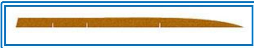
Next, cut one stringer with the notches. See "[Notches for Stringers and Frames](#)". In many cases, our stringers are made of two layers of plywood epoxy glued together. The joints are staggered, see the plans. In
