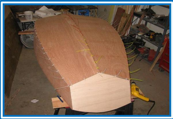
When installing the side panels, beware of longitudinal alignment. If the side panels seem not to fit, slide them back and forth. A small movement will bring everything into alignment. As is typical with our method, allow the panels to float, meaning that we try to attain fairness first. Use as little fasteners as possible and do not pull the panels against the frames unless absolutely necessary.
