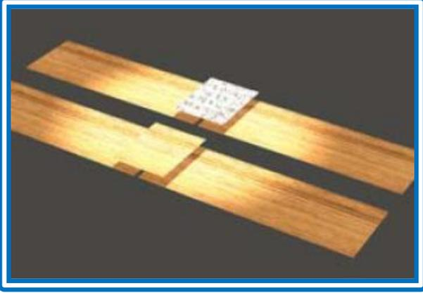
Once the jig is ready, cut the panels for the sides and bottom. The dimensions on our expanded panel drawings are very accurate so there is no need to use a safety margin. We suggest starting planking with the bottom panels. Cut the panels and use fiberglass splices to join the pieces of plywood. The plans or building notes specify the type of glass to use. The picture shows a butt block at the bottom and a fiberglass splice at the top. Note: No butt blocks needed if puzzle joints are used.
