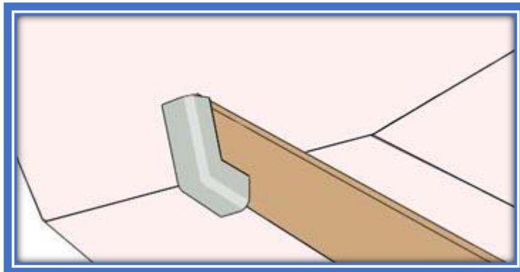
The stringers are always tabbed to the transom with the same type of glass and number of layers than the stringers to hull bottom.
