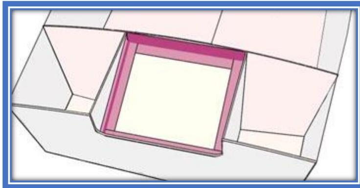
The bottom of the motorwell must be tabbed all around to the transom, motorwell sides and motorwell bulkhead.
