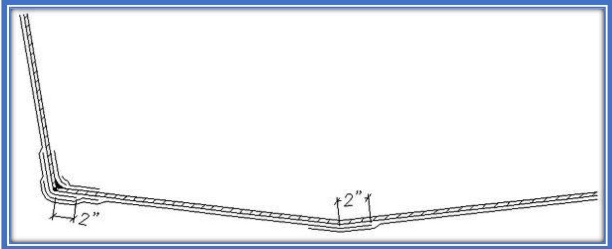
Extend the fiberglass tape and fabric beyond the corners and edges:
