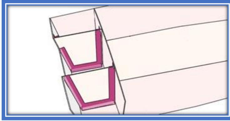
The motorwell sides play an important role in the structure of your boat. They must be fibreglassed to the motorwell bulkhead, the bottom panel and the transom with the same type of glass and number of layers than the stringers to the bottom.
