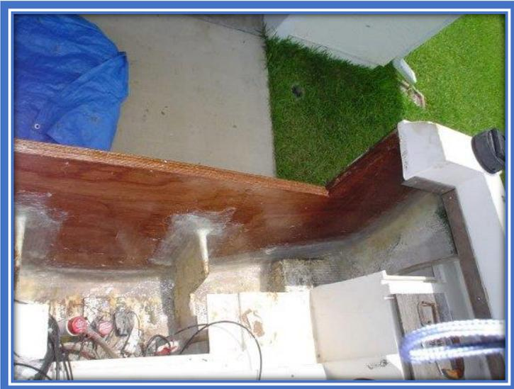
Here is the core tabbed into the hull (again, the stringer should not have been tabbed back in yet as in this picture).
