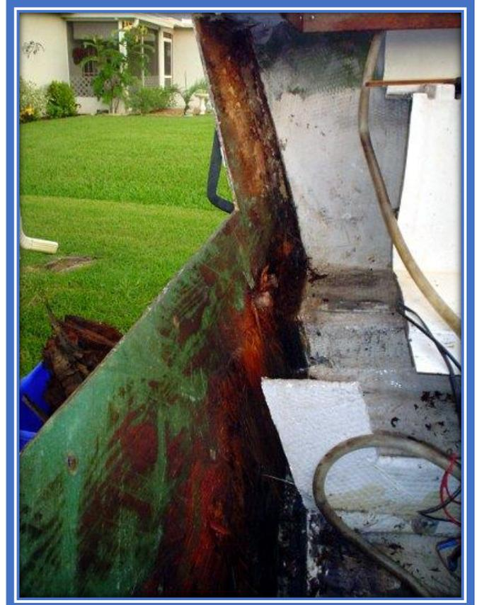
Once the old plywood and putty are removed, make a template of the transom using cardboard or cheap plywood (or anything else handy). You will use this template to cut your transom core and to draw/cut the wide fiberglass pieces that will make up the new inside transom skin.
