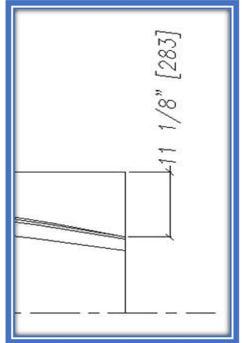
Also, on page E248/4, the camber for Station A was not positioned in the correct spot. It should be from the  $4 \frac{1}{2}''$  step to the sheer line. Which makes the camber  $1 \frac{1}{8}''$  [29].
