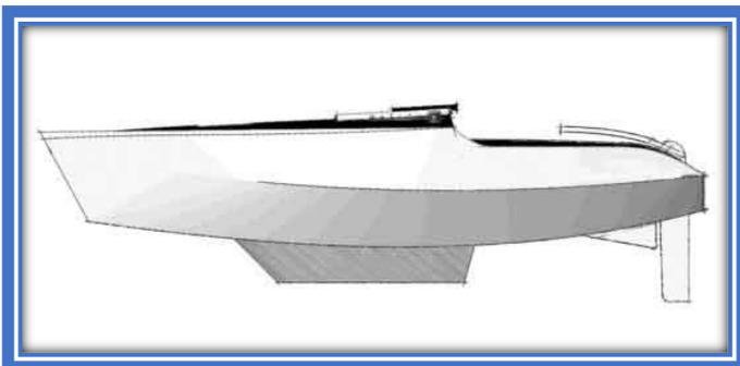
The rudder moves forward on the new transom and rotates in a slot just like in the VG20. The rudder gets better support and it will give better control in its new location. It can move up and down for shallow water sailing. The skeg became slightly larger for better tracking. The split backstay is connected to chainplates mounted on the new transom. The backstay moves to the new transom. This will limit the amount of roach in the main but that is perfect for long distance sailing.
